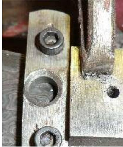
Start with two pieces of steel (here  $\frac{3}{4}$ " x  $\frac{3}{8}$ " x 2.0"). They just have to be thick enough not to bend easily (small angle iron would do), wide enough to drill and tap the bolt holes, and long enough to span the actual blade height plus room for the bolts. The bolts here are 8x32 socket cap screws. I used them because I have a box of a 100. I would not do lighter and anything over  $\frac{1}{4}$  is way overkill.
