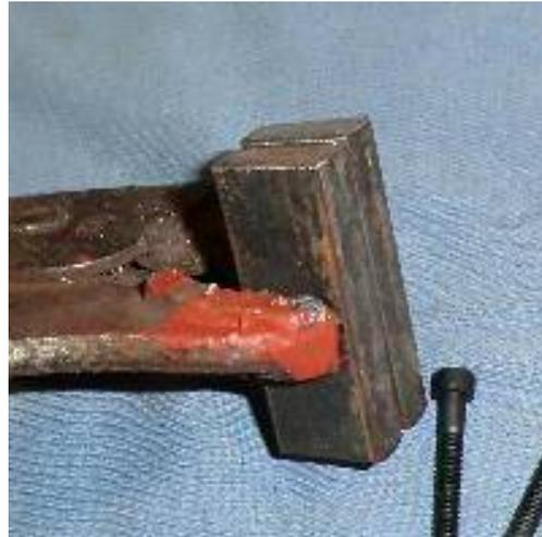
The first step is to drill two holes close to each end, hopefully near the center line and perpendicular to the surface. A cross-vise on the drill press makes this a whole lot easier. The size of the hole is controlled by the bolt selection. In this case a 8x32 bolt requires a #27 bit.
