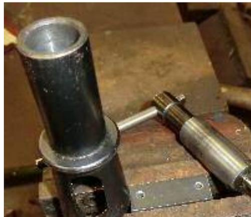
Next - bolt the pieces together and discover just how well you did in aligning the surfaces. You can fix any problems with a bit of care on the grinder or with a file but....
