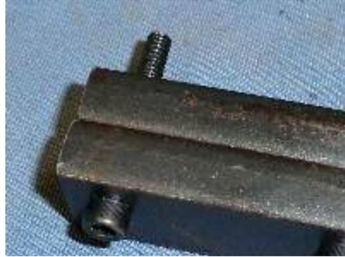
I have a mill (Series 1 Bridgeport clone) with a flood coolant system, so it's over to the mill to run a shallow cut to insure that both the front and back surfaces are precisely aligned.
