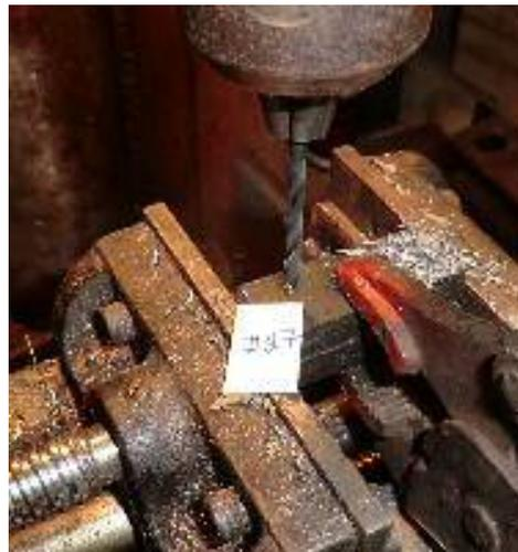
One of the pieces needs to be drilled so that the bolt passes easily through the piece. A free fit for an 8x32 bolt requires a #16 bit, so that is what is used here. As an additional benefit, the slop in the hole allows the camp to accommodate a taper in the blade profile.
